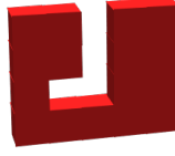
■ Figure 2 Example of a bent cavity, assuming that the planes on the sides into and out of the page were also filled in, leaving a single-cube-wide path into the interior of the shape.
